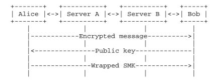
Figure 3: Delivering a Secure XMPP Message
