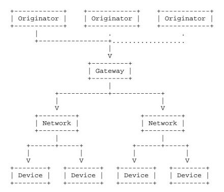
Figure 4: Delivering an Emergency Alert
