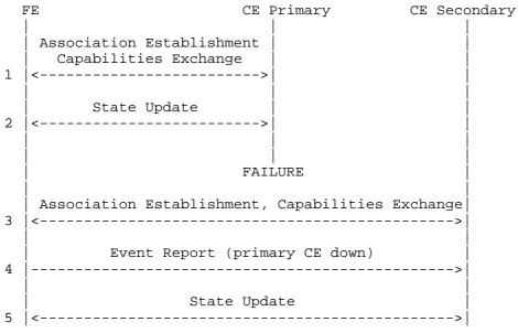
Figure 2: CE Failover for Cold Standby
