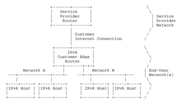
Figure 1: An Example of a Typical End-User Network
