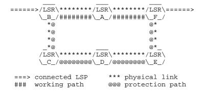
Figure 2: Steering Protection in an MPLS-TP Ring
