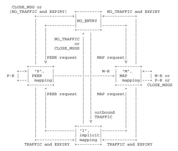
Figure 16: PCP State Diagram
