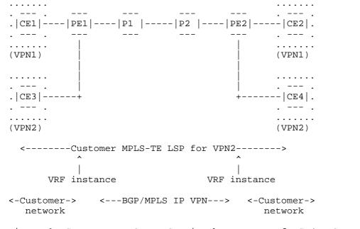
Figure 1: Customer MPLS TE LSPs in the context of BGP/MPLS IP VPNs
