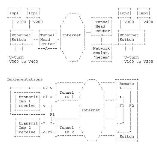
Illustrations of a test setup with a bidirectional tunnel. The upper diagram emphasizes the VLAN connectivity and geographical location. The lower diagram shows example flows traveling between two measurement implementations (for simplicity, only two flows are shown).
