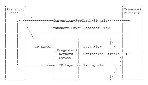
Figure 1: The ConEx Protocol in the Internet Architecture
