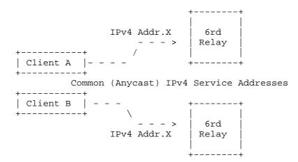
Figure 3: 6rd Anycast IPv4 Service Address Model
