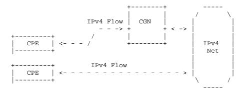
Figure 5: Overlay CGN Deployment
