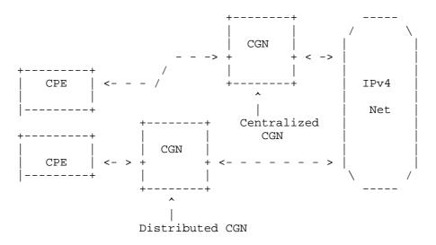
Figure 7: CGN Deployment: Centralized vs. Distributed
