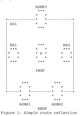
Abbreviations used: RR - Route Reflector P - Core router
