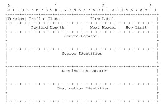
Figure 3.4: ILNPv6 Header as Seen by ILNPv6-Enabled End-Systems
