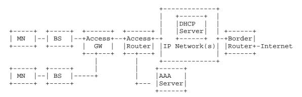
Figure 1: Key Elements of a Typical Cellular Network
