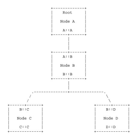
Figure 32: Storing Mode with Node-Owned Prefixes
