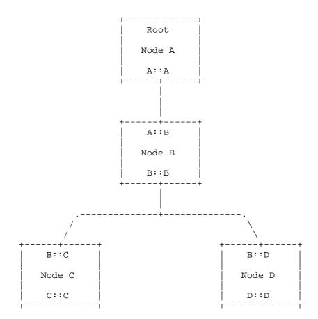
Figure 34: Non-Storing Mode with Node-Owned Prefixes
