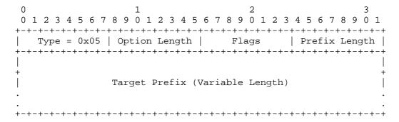
Figure 25: Format of the RPL Target Option
