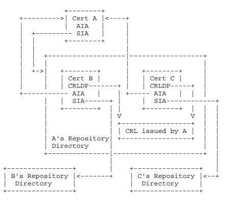
Figure 1. Use of AIA and SIA Extensions in the RPKI
