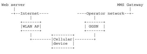
A Cellular Device with Two Network Interfaces
