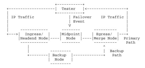
Figure 2. System Under Test (SUT) for Sub-IP Node Protection
