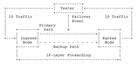
Figure 4. System Under Test (SUT) for Sub-IP Local Link Protection
