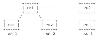
Consider the example given above, where (PE1, CE1) and (PE2, CE3) sessions are iBGP. In BGP/MPLS VPNs, a route received from CE1 above may be distributed to the VRFs corresponding to the attachment points for CEs 2 and 3.
