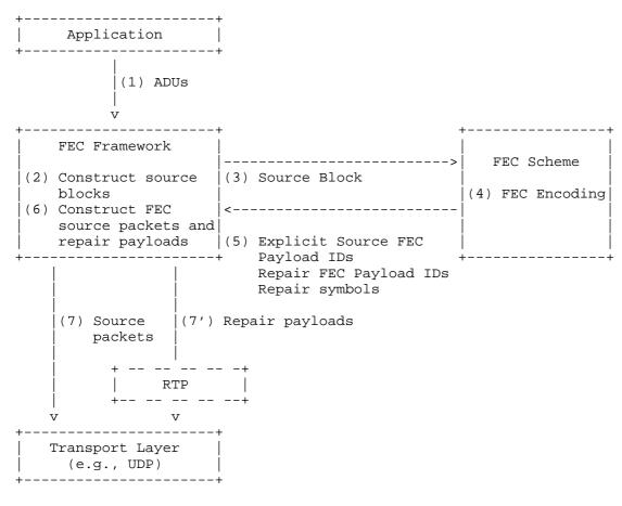
Figure 3: Sender Operation with RTP Repair Flows
