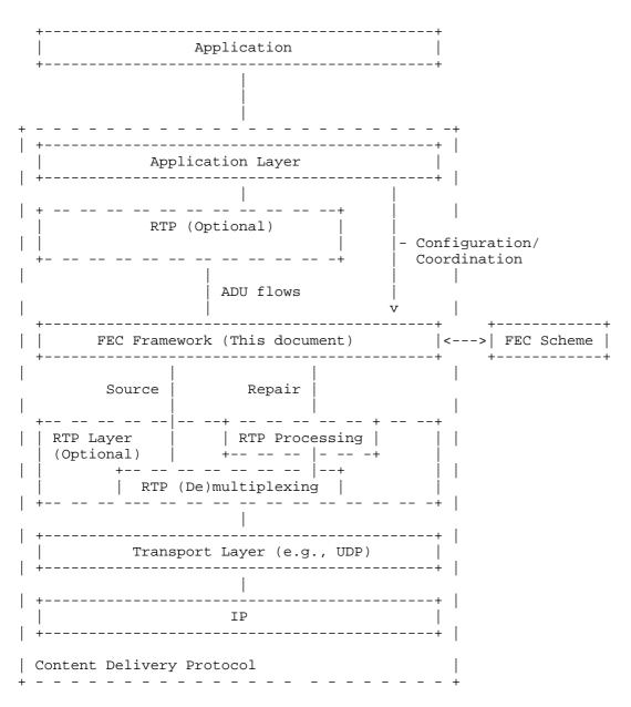
Figure 1: FEC Framework Architecture
