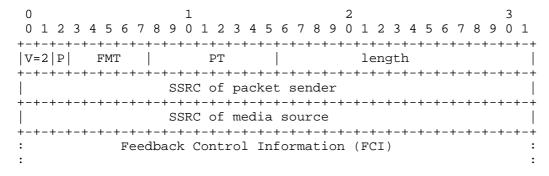
Figure 4: The Common Packet Format for the RTCP Feedback Messages
