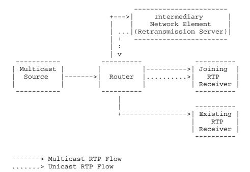
Figure 1: Rapid Acquisition through an Intermediary Network Element
