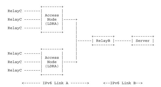
For example, if a client sent a DHCP Solicit message that was relayed by RelayC and the LDRA to another relay agent, RelayB, and then to the server, the server would receive the following Relay-Forward message:
