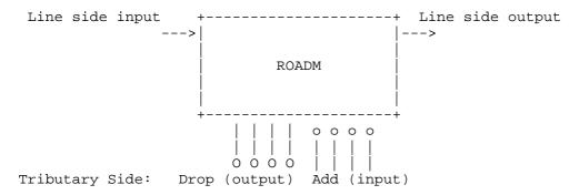
Figure 1. Degree-2 Unidirectional ROADM
