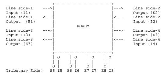
Figure 2. Degree-4 Bidirectional ROADM
