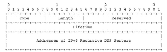
Figure 1: Recursive DNS Server (RDNSS) Option Format
