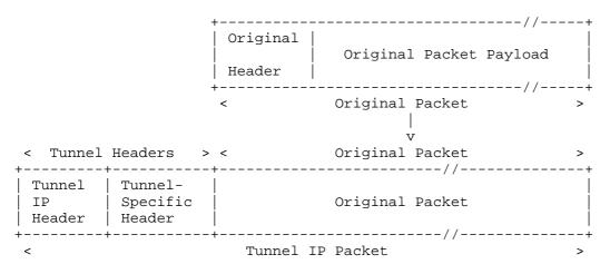
Figure 2: IP Tunnel Encapsulation
