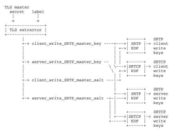
Figure 1: The derivation of the SRTP keys.
