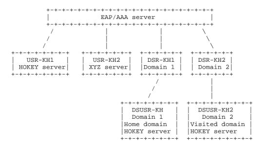
Figure 1: Example Key Delivery Architecture for the Different KRS and  $_{\mbox{\scriptsize KDS}}$
