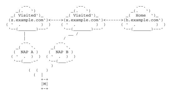
Figure 1: Example roaming scenario with intermediating realms. The mobile host authenticates to the home realm through one or more visited realms.
