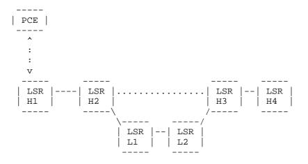
Figure 6: Higher-Layer Signaling Trigger Model
