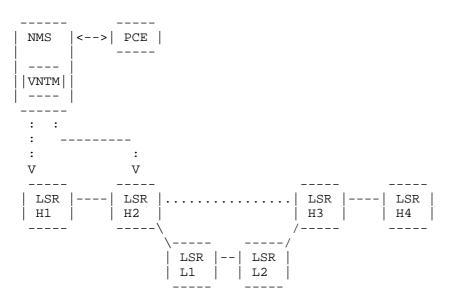
Figure 8: NMS-VNTM Cooperation Model (integrated flavor)
