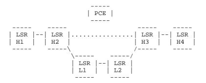
Figure 2: Single PCE Inter-Layer Path Computation
