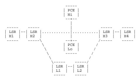
Figure 3: Multiple PCE Inter-Layer Path Computation with Inter-PCE Communication
