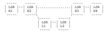
Figure 1: A Simple Example of a Multi-Layer Network
