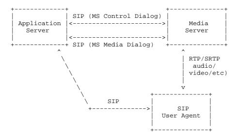
Figure 1: Basic Signaling Architecture
