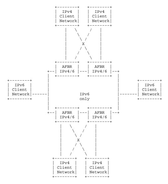
Figure 2: IPv4-over-IPv6 Scenario
