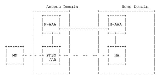
Figure 2: CDMA2000 Packet Data Network Architecture with Mobile IPv6
