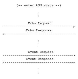
Figure 3: CAPWAP Control Protocol Exchange
