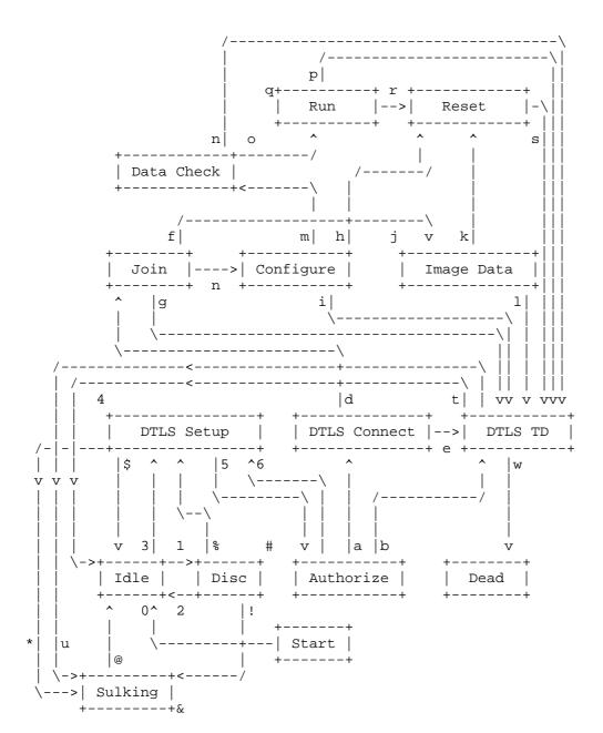
Figure 4: CAPWAP Integrated State Machine
