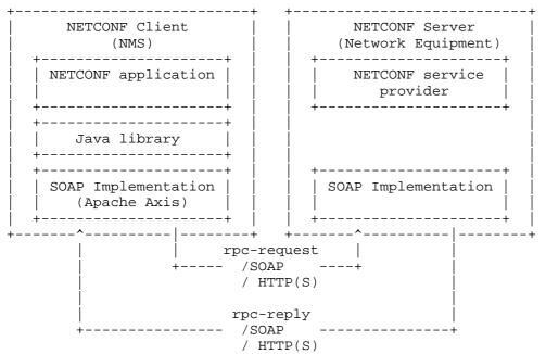
Figure 2: Architecture of NETCONF Implementation Using SOAP
