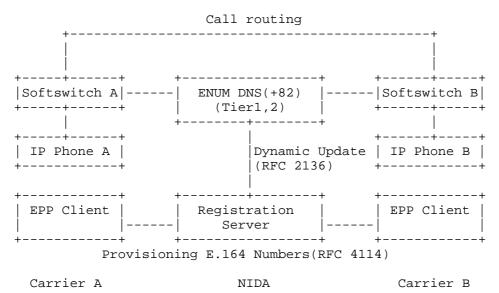
Figure 1: Infrastructure ENUM Trial System Topology
