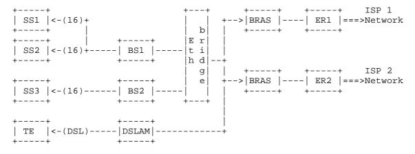
Figure 5: Integration of 802.16 Access into the DSL Infrastructure
