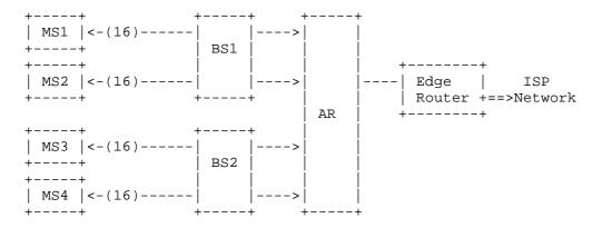
Figure 3: Point-to-Point Link Model
