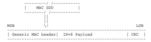
Figure 3: IPv6 encapsulation
