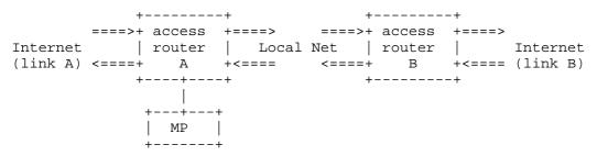
Figure 4: Perimeter Metering Process Position
