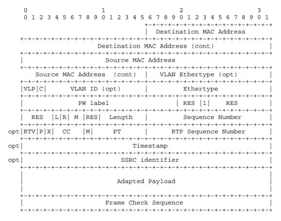
Figure 6. TDMoIP Packet Format for Ethernet
