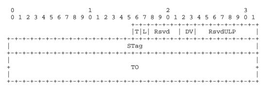
Figure 4: Tagged Buffer DDP Header
