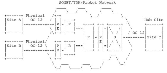
Figure 13: SONET Interconnect Emulation Example Diagram
