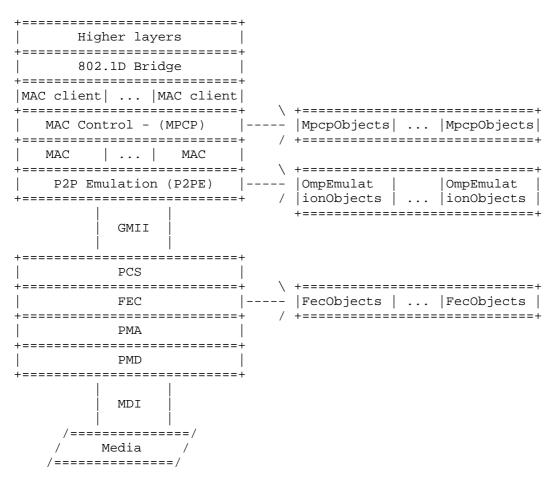
The association is straightforward for the ONU interface. There is one logical and one physical interface, and a single copy exists for each layer that can be remotely queried by the OLT.
