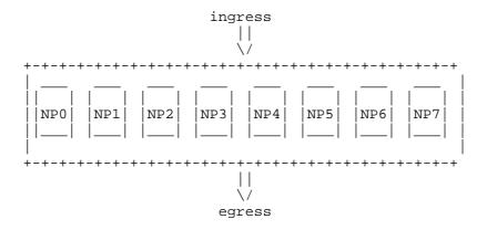
To assign incoming traffic to the various NPs, suppose a hashing algorithm performs an exclusive-or (XOR) operation on the least significant 3 bits of the source and destination MAC addresses in each frame. (This is an actual example the authors have observed in multiple devices from multiple manufacturers.)
