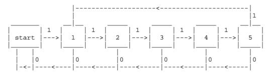
Initially, we begin in the "start" state. A "1" bit moves us into the next highest state, and a "0" bit returns us to the start state. From state 5, a "1" bit takes us back to the 1 state and a "0" bit returns us to "start".
