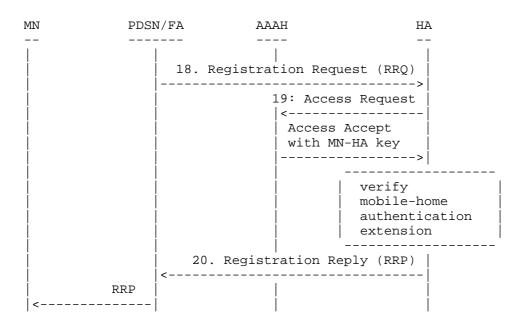
Figure 4. DMU Procedure Flow (part 3)
