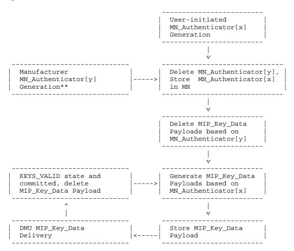
Figure 3. MN\_Authenticator and MIP\_Key\_Data Payload State Machine
