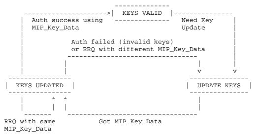
Figure 6. RADIUS AAA Server DMU State Machine
