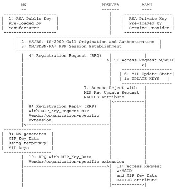
Figure 4. DMU Procedure Flow (part 1)
