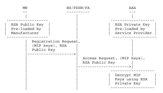
Figure 1. RSA Encrypted Key Distribution
