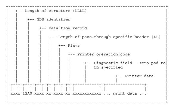
Figure 3. Layout of the printer pass-through header
