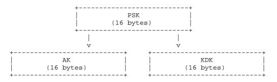
Figure 2: Derivation of AK and KDK from the PSK
