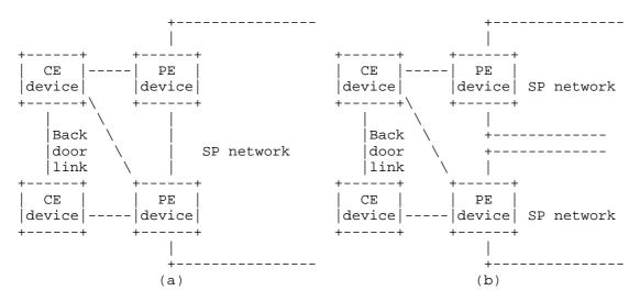
Figure 4. Combination of Dual-Homing and Backdoor Links for CE Devices
