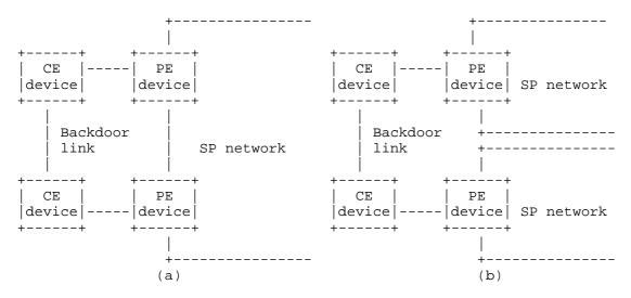
Figure 3. Backdoor Links Between CE Devices
