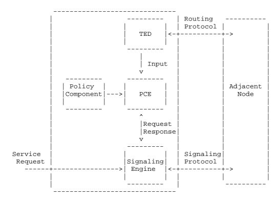
Figure 6. Policy Component in the Composite PCE Node
