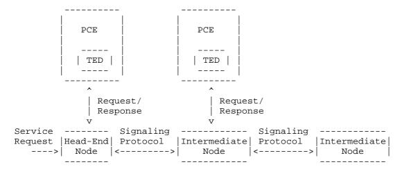
Figure 3. Multiple PCE Path Computation
