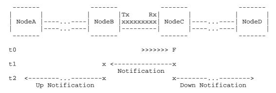
Figure 1: Uni-directional failure detection
