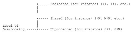
Also, when using shared recovery, one may support preemptible extratraffic; the recovery mechanism is then expected to allow preemption of this low priority traffic in case of recovery resource contention during recovery operations. The following sections will consider the above-mentioned overbooking options when analyzing the different recovery mechanisms.
