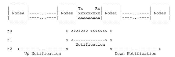
Figure 2: Bi-directional failure detection
