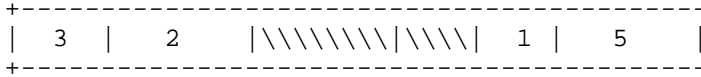
Figure 3.10. The codebook memory, length lMem=147 samples, and the target vector 5, length 40 samples.
