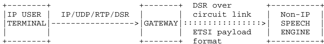
c) IP user terminal to non-IP speech engine via a gateway
