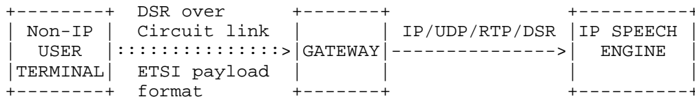
b) non-IP user terminal to IP speech engine via a gateway
