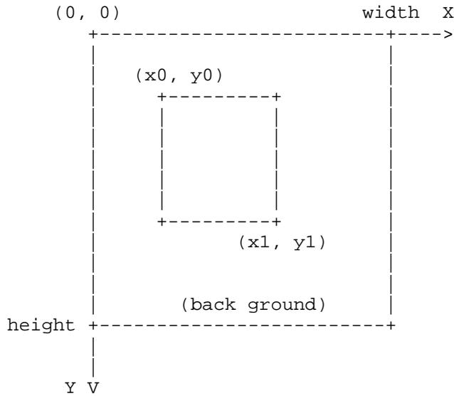
The parameter action indicates how the two images are merged. If it set to 0, The second image is simply overlaid on the back ground image. On the other hand any non-zero value
