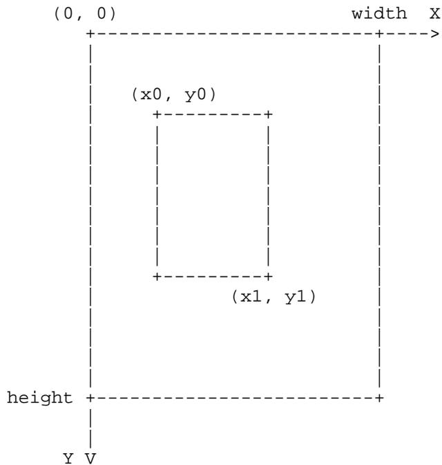
As can be seen in the diagram, the rectangular area to be extracted is specified by the parameters x0, x1, y0, y1, which are decimal strings.
